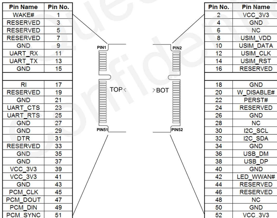
Figure 2: Pin Assignment
