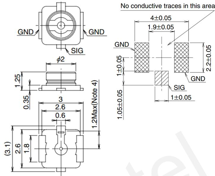
Figure 13: Dimensions of the RF Connector (Unit: mm)
