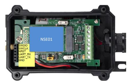
Connection: USB TTL GND <----> GND USB TTL TXD <----> UART\_RXD USB TTL RXD <----> UART\_TXD
