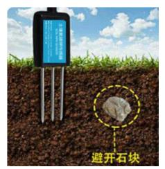
Choose the proper measuring position. Avoid the probe to touch rocks or hard things. Split the surface soil according to the measured deep. Keep the measured as original density. Vertical insert the probe into the soil to be measured. Make sure not shake when inserting.
