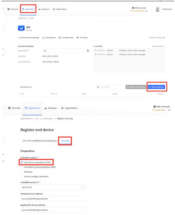
For this device, set up to use Cayenne payload, so TTNV3 can parse the sensor data properly.
