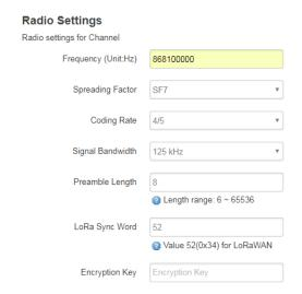
This parameters set is for uplink (receive data for LoRa End Node). According to LoRaWAN spec, the downlink radio parameters frequency is defined by network server (TTNV3). LG01-N will adjust downlink parameters according to info from TTNV3.
