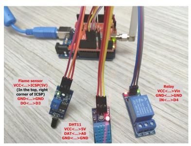
There are three sensors connect to the LoRa Shield + UNO. These sensors are flame sensors, DHT11 (Temperature & Humidity sensor) and Relay. Please use the connection as we show in the photo.
