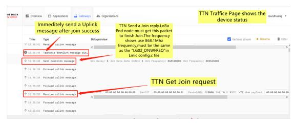
Note: The LG02\_DNWFREQ value in Arduno\_LMIC/src/Imic/config.h should match downlink frequency from
