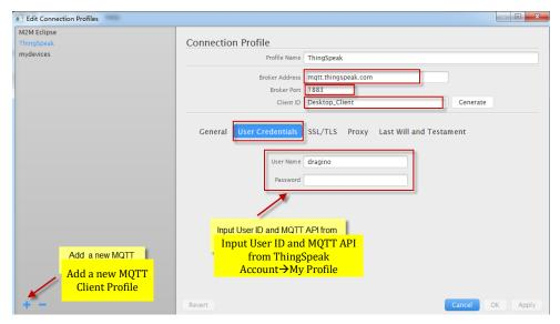
After add the profile, connect it and publish to the corresponding Channel with correct API key. MQTT API see this document:
