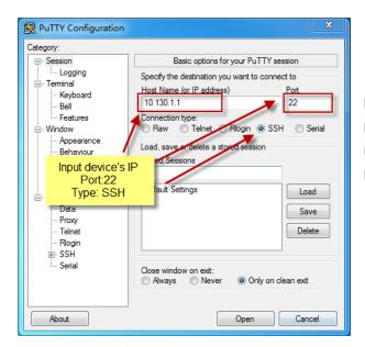
IP address: IP address of LG01-N
