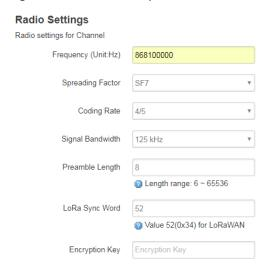
This parameters set is for uplink (receive data for LoRa End Node). According to LoRaWAN spec, the downlink radio parameters frequency is defined by network server (TTN). LG01-N will adjust downlink parameters according to info from TTN.
