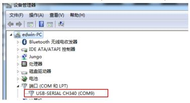
After install the driver, start Arduino and we will be able to use the board Arduino UNO and corresponding COM port to program UNO now.
