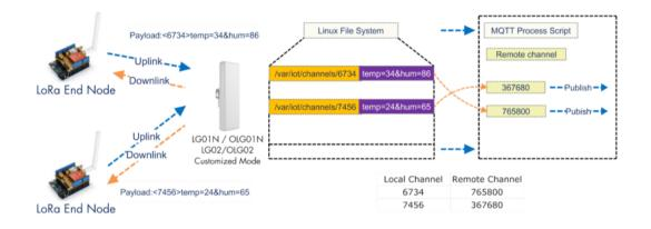
The above diagram shows an overview of how the end to end messaging system works, from the creation of a message in a LoRa End Node (typically a remote sensor device) to the publishing of the message on a host IoT Platform such as ThingSpeak, AWS or Azure via the MQTT protocol.
