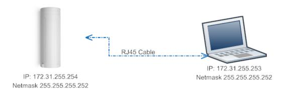
The DLOS8 has a fall-back IP address on its WAN port. This IP is always enabled so you can use the fall-back IP to access DLOS8 no matter what the WiFi IP is. The fall back IP is useful for connecting and debug the unit.
