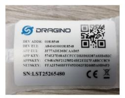
Note: You may be able to change these codes in a device by using a configuration facility on the device e.g. the LT-22222 uses a serial port access and a series of AT commands. Changing the codes may be necessary in the case where you have to use codes assigned by a LoRa WAN server.
