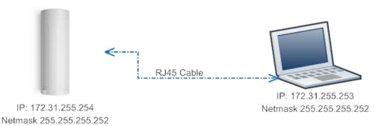
The DLOS8 has a fall-back IP address on its WAN port. This IP is always enabled so you can use the fall-back IP to access DLOS8 no matter what the WiFi IP is. The fall back IP is useful for connecting and debug the unit.
