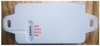
Use a metal wire to short NRST and GND pin will reset the LHT65.
