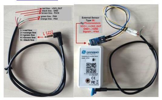
User can also connect PA9 and PA10 together, with these two pins shortcut, LHT65 will know if the probe is connected well in the socket.
