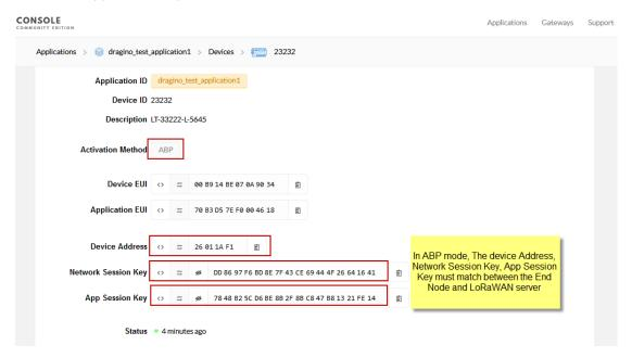
Note: user just need to make sure above three keys match, User can change either in TTN V3 or Device to make then match. In TTN V3, NETSKEY and APPSKEY can be configured by user in setting page, but Device Addr is generated by TTN V3.
