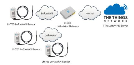
Assume the LG308 is already set to connect to <u>TTN V3 network</u>. We need to add the LHT65 device in TTN V3:
