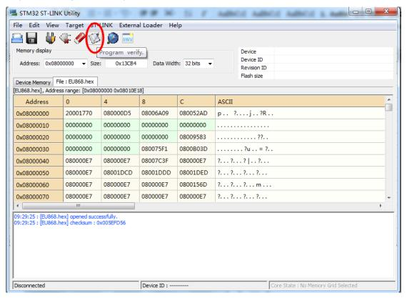
**Step5:** The led on the ST-LINK adapter will now blinking, click program verify button to select the image to be upgraded.
