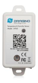
The Dragino LHT65 Temperature & Humidity sensor is a Long Range LoRaWAN Sensor. It includes a **built-in SHT20 Temperature & Humidity sensor** and has an external sensor connector to connect to external sensors such as **Temperature Sensor**, **Soil Moisture Sensor**, **Tilting Sensor etc**.
