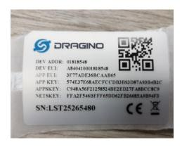
Note: You may be able to change these codes in a device by using a configuration facility on the device e.g. the LT-22222 uses a serial port access and a series of AT commands. Changing the codes may be necessary in the case where you have to use codes assigned by a LoRa WAN server.
