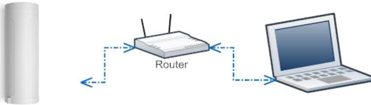
Alternatively, connect the DLOS8 Ethernet port to your router and DLOS8 will obtain an IP address from your router. In the router's management portal, you should be able to find what IP address the router has assigned to the DLOS8. You can also use this IP to connect.
