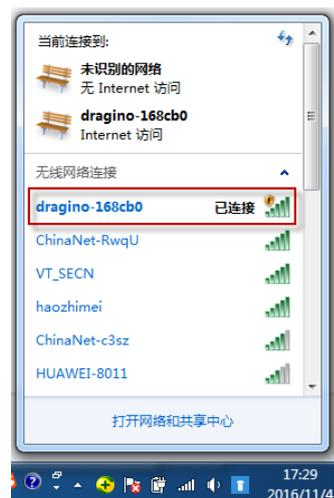
User can use a PC to connect to this WiFi network. The PC will get an IP address 10.130.1.xxx and the DLOS8 has the default IP [10.130.1.1](#)
