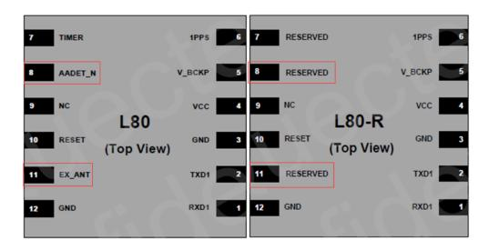
Figure 1: Different Pins between L80 and L80-R
