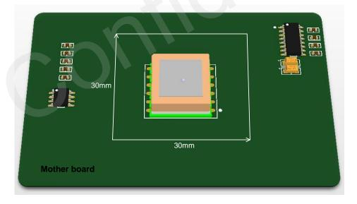
Figure 3: Recommended Ground Plane
