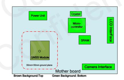
Figure 5: Recommended Placement of GNSS Module
