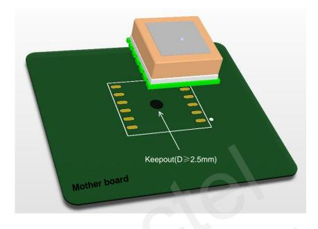
Figure 2: Recommended Keepout Area on Mother Board
