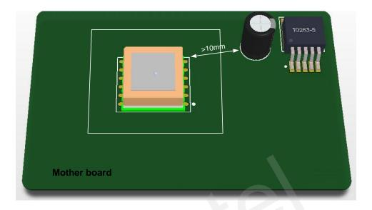
Figure 4: Recommended Distance between GNSS Module and Tall Metal Components
