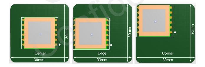
Figure 8: Test Board of Placement
