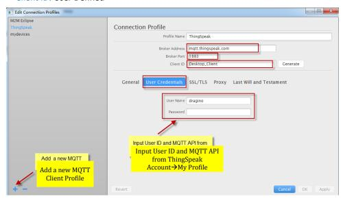
After add the profile, connect it and publish to the corresponding Channel with correct API key.
