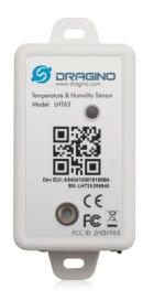
The Dragino LHT65 Temperature & Humidity sensor is a Long Range LoRaWAN Sensor. It includes a **built-in SHT20 Temperature & Humidity sensor** and has an external sensor connector to connect to external sensors such as **Temperature Sensor**, **Illumination sensor**, **Interrupt Sensor**, **ADC sensor etc**.
