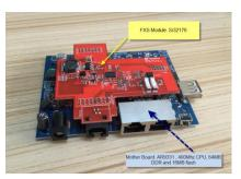
The DT01 is an offshore Open Source VoIP Asterisk appliance. It was composed by the MS14-P mother board and FXS module.
