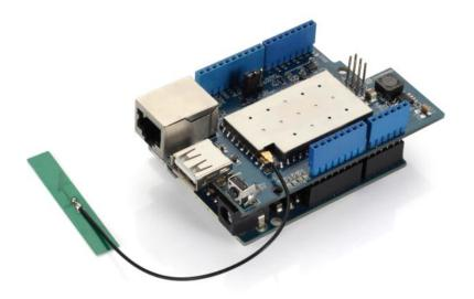
The Yun Shield made by Dragino HE module is the most powerful shield for Arduino. it provides easy internet connection for Arduino and also provide a 400Mhz OpenWrt system to Arduino.
